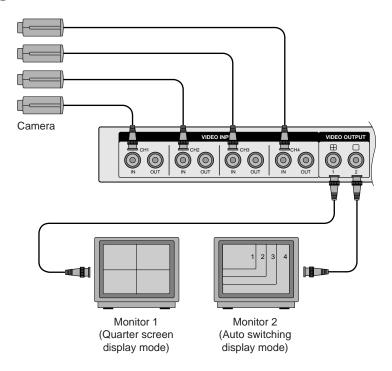
If you connect a monitor to the VIDEO OUTPUT terminal with the "  $\square$ " mark, it is configured as a quarter screen display. If you connect a monitor to the VIDEO OUTPUT terminal with the "  $\square$ " mark, it is configured as a quarter-section screen, single screen or an automatic sequence screen.
